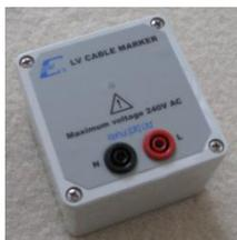
**LV Cable Marker** provides a means of identifying known points along a cable to simplify interpretation of TDR traces and/or to improve the accuracy of distance to fault determination. The unit is line powered and appears on the TDR trace like an intermittent fault but without interrupting supplies to customers.
